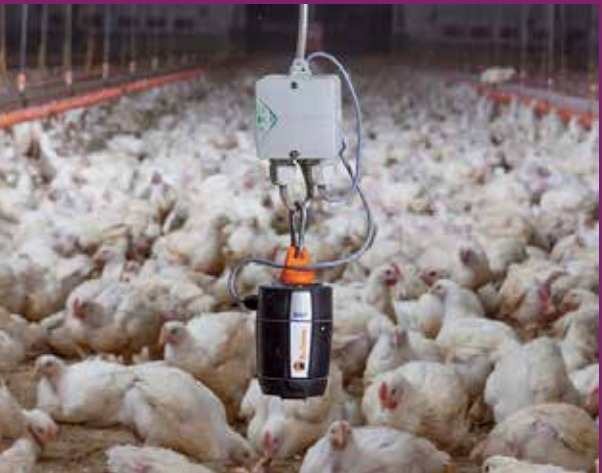
Ammonia meters can be an effective tool to monitor air quality. PHOTO CREDIT: BIG DUTCHMAN.
